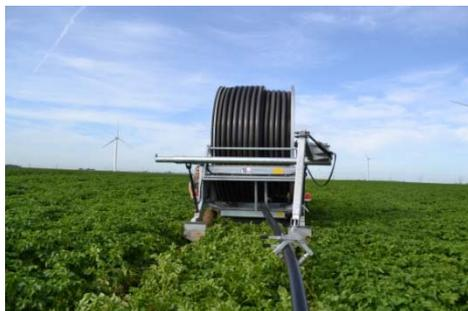
Now, the PE-pipe can be laid down along the line.
