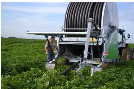
Swivel the swivel arm with the open fairlead with the help of the hydraulics over the PE-pipe and then lay down the PE-pipe.
