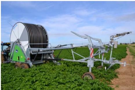
Lower the cart with the hydraulic cart lift and fix it to the ground.
