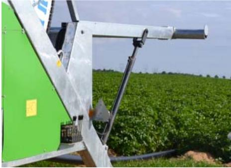
The hydraulic cylinders of the cart lift must be completely retracted in order to ensure the right position for the cart intake.
