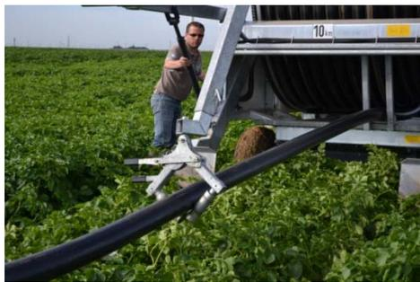
Move the PE-pipe with the hydraulic swivel arm into the desired position.
